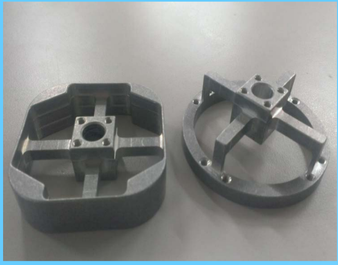
6 and 4-axis force/torque sensors design, Calibration machine
