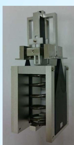
Nonlinear spring and rotor types energy harvester for TPMS, Prototypes
